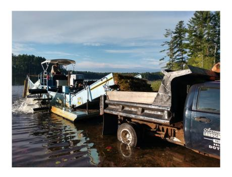
Fig. 1 - The Weed Harvester loading the truck with Fanwort
